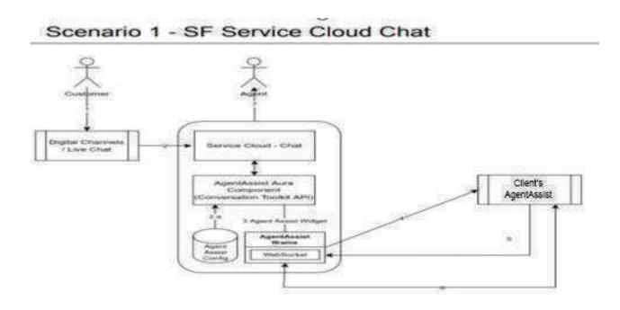
In this scenario, when a customer initiates a chat request in Service Cloud, the AgentAssist Aura Component is activated. This component serves as a bridge between Service Cloud chat and the Client's AgentAssist Engine. The process involves:
