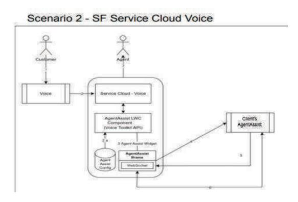
In this scenario, when a customer calls the contact center phone number and the Agent accepts the call via Service Cloud Voice, the AgentAssist Aura Component is triggered. This component serves as a link between Service Cloud Voice and Client's AgentAssist, executing the following steps:
